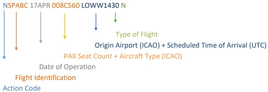
**For an arrival slot, there is NO blank between the action code and the flight identification.**
