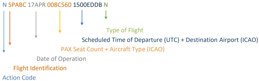
**For a departure slot, there is A BLANK between the action code and the flight identification.**
