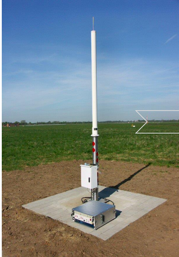
GPS L1 reference antenna GPS reference receiver (4x)
